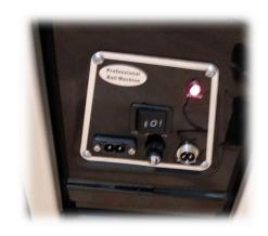
Once the battery is loaded, simply disconnect the DC wire and set the switch to "I" position.
